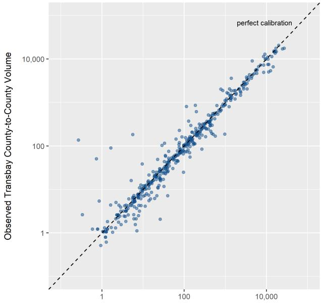
Figure 5-1. Transbay Auto OD Calibration Plot<sup>25</sup>
